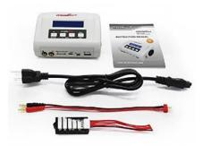
Your Cuta-Copter comes with a UP100AC *plus* charger. The charger is specifically designed to charge multi-cell batteries. The charger monitors charging through each cell of the battery with a `balancing cable'.
